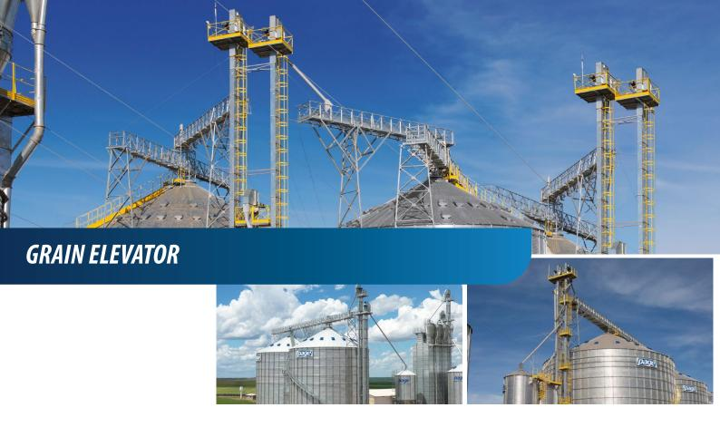
The bucket elevators Pagé are designed to work in vertical position of solid bulk in continuous operation. Totally made of galvanized steel sheet, the capacity can vary from 5 to 1,500 ton/hour and the electrical drive is by gearmotor
